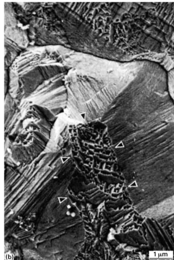
Figure 2 As-plated surface morphology of samples deposited at or above 0.01 A cm -2 , "truncated-pyramidal" structures. The ridged terraces, perpendicular to the growth direction, are outlined by arrows in (b).
